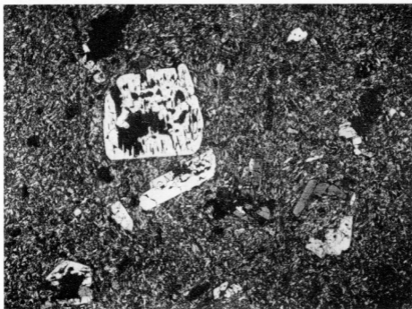
Fig. 2. Trachyandesite with stray phenocrysts of a Na-rich plagioclase in a fine grained paste of alk. feldspar microlites with trachytoidal texture. Mafic minerals as pseudomorphs. Los Ajaches, N fr. P. Papagayo, Lanzarote.
