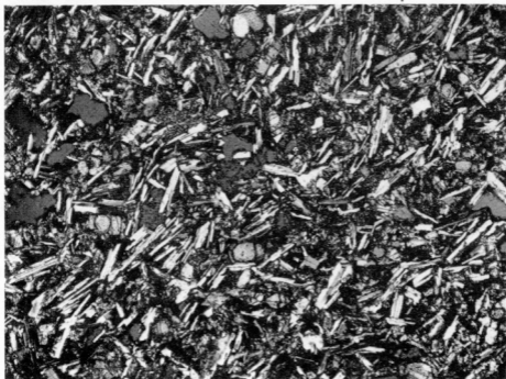
Fig. 1. Olivine basalt (plagioclase-rich) with sparsely phenocrysts of olivine and augite in a paste consisting of plag., augite and ore. Quaternary lava at Puerto Naos, to the north from Arrecife, Lanzarote.
