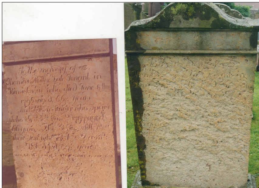
Grave of Thomas Miller (1729-1795) & Alison Sinclair (1730-1797) showing erosion and loss of text.
