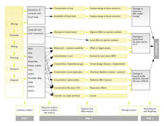
Figure 4. Detailed representation of damage model in the Eco-indicator 99 methodology (step 2).
