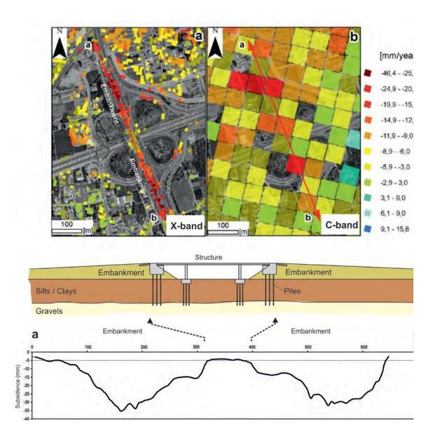
**Figure 2.** (Above) Subsidence rate map of a highway bridge derived from X-band and C-band satellite images. (Below) Bridge scheme and subsidence profile along the bridge axis (adapted from Herrera et al., 2010).
