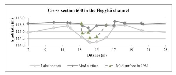
Figure 3: A cross-section of the Hegykő channel.
