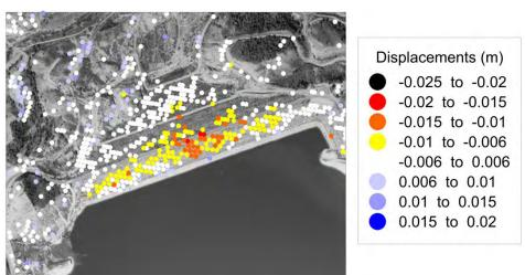
Figure 1. (Above) 1993-2009 displacement map derived from ERS and ENVISAT high resolution images (regional analysis). Note the deformations detected on the lower-right corner of the map corresponding to La Pedrera Dam. (Below) Individual analysis of La Pedrera Dam using very high resolution TSX images from 2008 to 2010.
