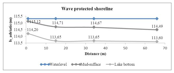
Figure 4: A cross-section of the shoreline in a wave protected area.
