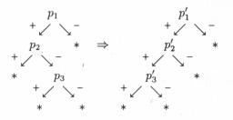
The encoding Enc(B) of B may be found from that of A by interchanging in Enc(A) the second and third component in the block determined by p. **Example**: If A is encoded by  $Enc(A) = (p_1(p_2 * (p_3 * *))*)$  then (if switch is applied in  $p_2$ ), we find for B the encoding  $Enc(B) = (p_1(p_2(p_3 * *)*))*)$ .
